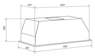
\* allow 5mm clearance for installation
