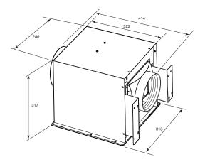
Remote fan motor goes into ceiling space. NOTE: Check that you home has a ceiling space above the kitchen to locate the motor.
